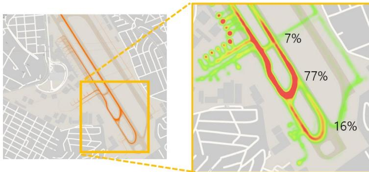
This is from an investigation into aircraft taxiing practices at an airport. Aside from showing the volume of traffic that uses each of the runway entry points, the image demonstrates another use of data, somewhat removed from investigation. The image shows that one of the three runway entries is being used far less frequently than the others. This could allow the airport to refine its maintenance planning and focus more on the two that are used more frequently.
