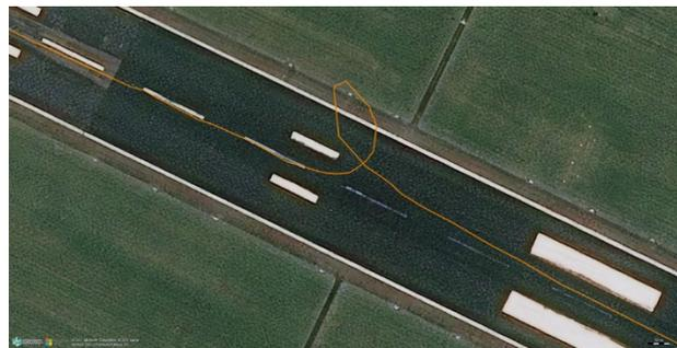
These two images show the path of fire vehicles. The track shows that the vehicle does not follow the hard surface but cuts across the grass; there is data validation required here to confirm that the track is accurate. The very straight line across the grass suggests that data was not collected correctly and the gap was filled in by the software. This may be an example of a blind spot that the ADS-B ground receiver at an airport or just a momentary loss of data.
