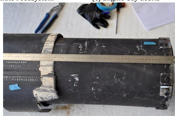
(e) Combustion chamber region where fins were attached
