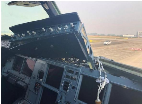
40 min after take-off, while in cruise (FL321), the RH windshield of this A319 separated. An immediate descent towards a lower altitude was conducted, followed by a diversion to the nearest airport (Chengdu, China), where an uneventful landing was performed.
