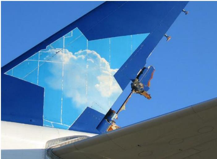
During this event, the rudder was lost due to weakening of its structure (composite sandwich disbonding leading to reduced torsional stiffness).
