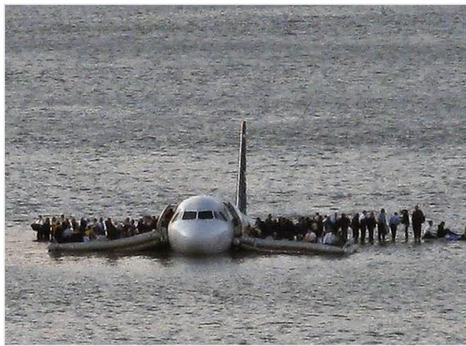
This aircraft encountered a flock of birds after take-off, resulting in multiple bird strikes impacting both engines, with subsequent significant loss of thrust on both engines.
