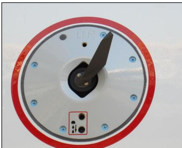
This A330 experienced a blockage of all 3 Angle-of-Attack (AoA) probes. They were fitted with a new configuration known as the conic plates.
