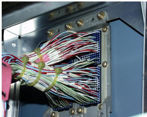
The root cause of this event was that one flight control computer (ELAC) input wires had been inverted during maintenance. This resulted in the Captain's sidestick to be inverted in roll.
