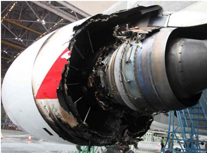
This A380 aircraft experienced an Intermediate Pressure Turbine (IPT) disc failure to engine #2 during climb.
