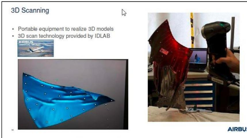
The scanned data allowed an assessment of which parts had been recovered and which remain on the ice sheet. A 3D reconstruction was produced which allowed an insight of how the engine event may have unfolded.
