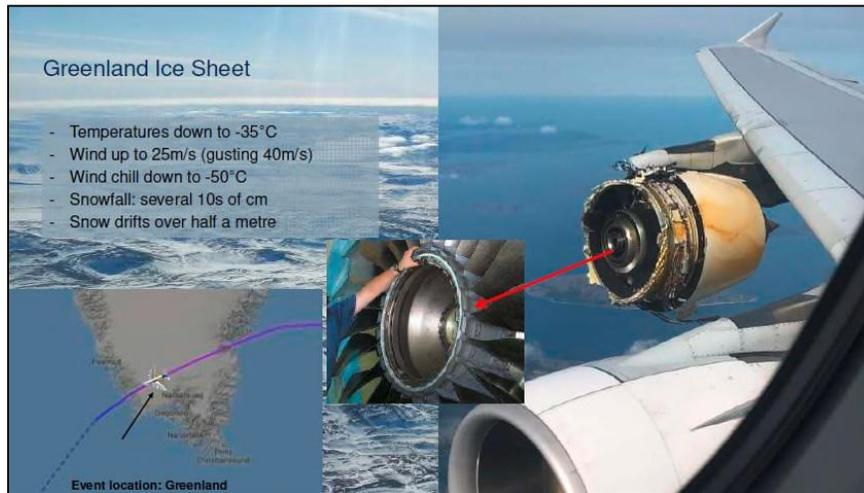
Retrieval of the engine components is crucial to understanding the root cause, the key component of interest being the fan hub, a 250kg piece of titanium 80cm in diameter. The fan hub is the central rotating component to which the fan blades are attached. The investigation team faced a huge challenge due to the geography and the extreme climatic weather and looked to technology to help search for the fan hub.
