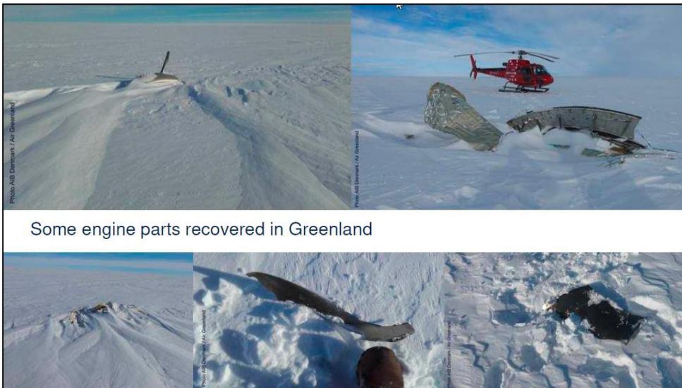
As the fan hub had not been located, the investigation team needed to ensure that maximum data was extracted from these recovered parts. The data would also support any hypothesis put forward and validate any analysis.
