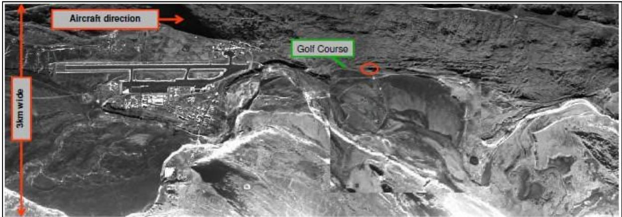
Examination of the image confirmed that the test piece had been detected, indicated by a bright white return on the radar image. A second radar return was seen on the image in the vicinity of the test piece. The cause of this return was not known and when the team returned to the site, we discovered metallic fencing wire buried under the snow.
