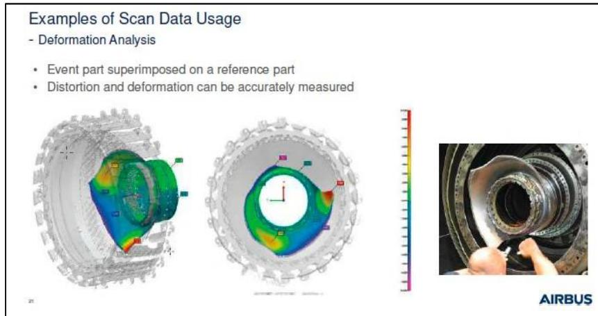
Advantages of the 3D scanning is that it provides an accurate record of parts as they were recovered and before any disassembly or destructive testing. The data can be made available to all parties of the investigation so that analysis can begin simultaneously. The data can be imported into Catia or viewed as a 3D pdf model.
