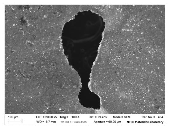
**Figure 16**. Hole in the bottom of the copper foil adjacent to the aluminum protrusion in figure 15, cell 6.
