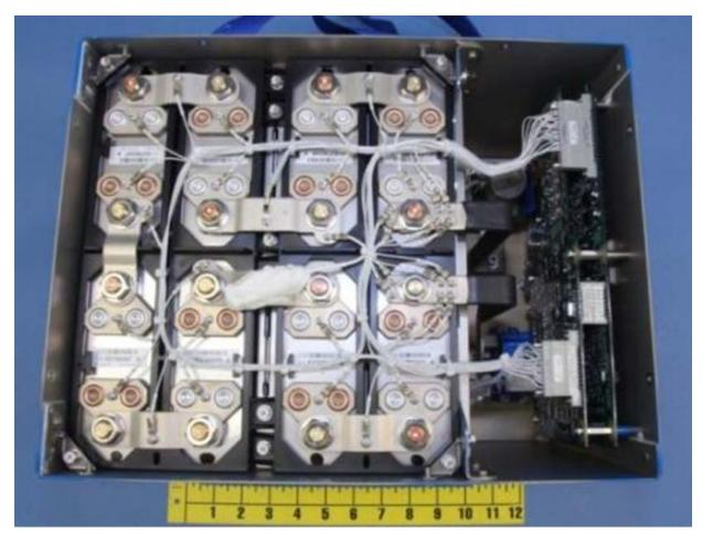
Figure 1. Exemplar for the 787 main and APU batteries.
