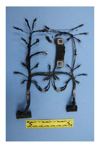
Figure 10. Wiring harness, as removed. (View is from the bottom.)
