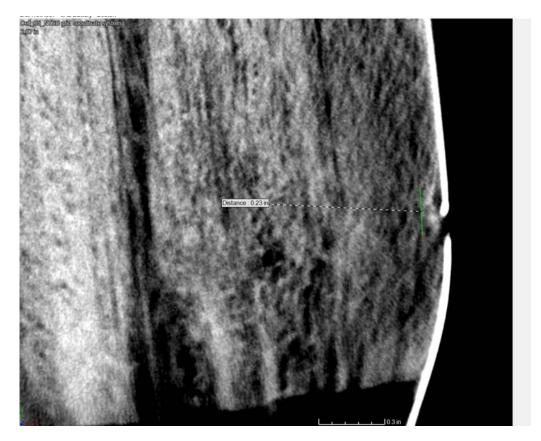
Figure 11. CT scan of cell 5 showing breach in case.
