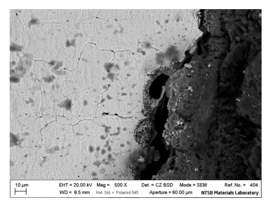
Figure 14. Grain boundary decohesion near a foil hole, cell 6.
