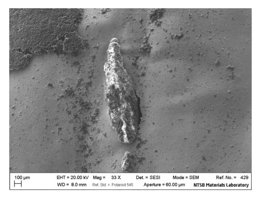
Figure 15. Aluminum lump projecting through the bottom of a copper foil wrap, cell 6.
