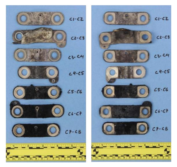
**Figure 7**. Views of bus bar contact surfaces. The photo on the left shows the contact surfaces facing the washer and the nut. The photo on the right shows the contact surfaces facing the battery terminal.
