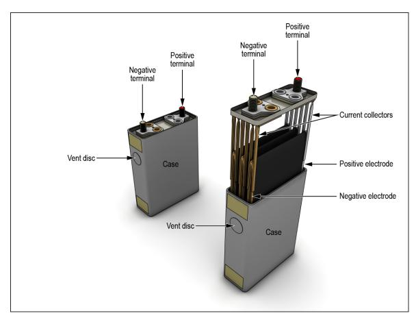
Figure 3. Cell design with three internal electrode winding assemblies.
