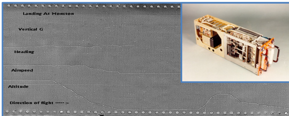
Figure 1: 1953 era foil flight data recorder, designed exclusively for accident investigation.
