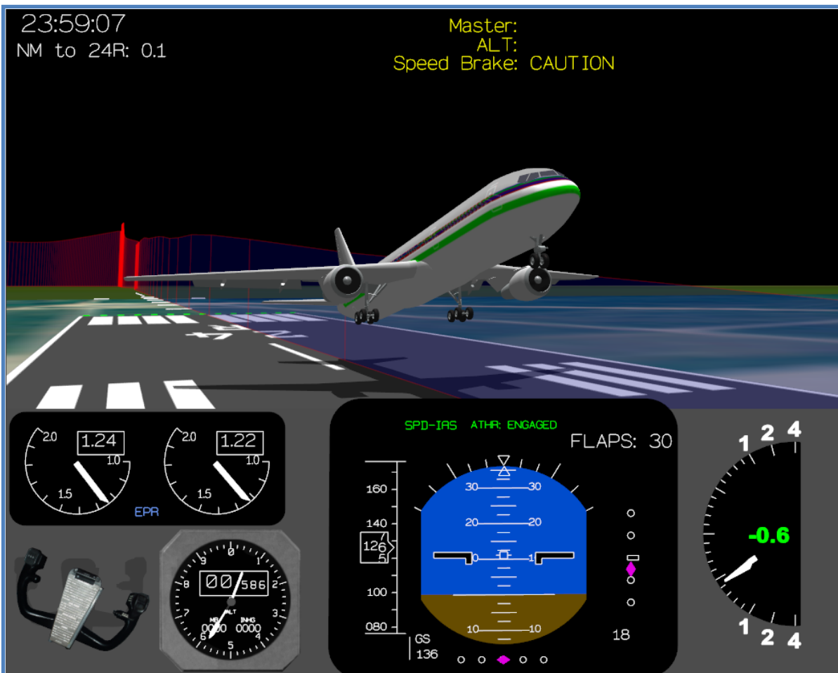
Figure 5: B757 landing with Speed Brakes extended resulting in tail contact and hard landing
