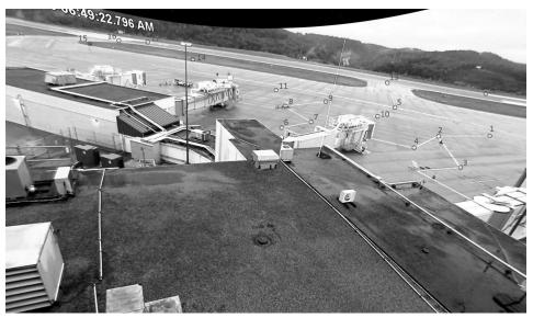
Figure 11. Accident area with superimposed ground track and azimuth direction from the parking garage camera to the airplane.
