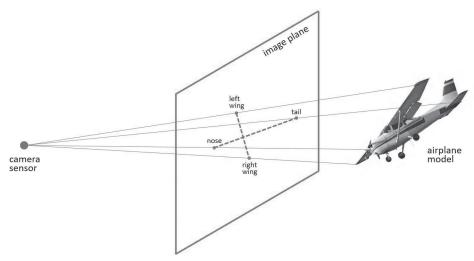
Figure 2. Projection from 3-D field of view onto a 2-D video frame.
