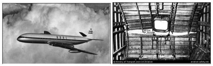
Figure 3. de Havilland Comet window failure.
