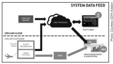
Figure 1: QAR data processing for both mobile service and FDM program.
