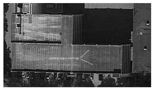
Figure 6. Parking space marking lines used for calibration of garage camera video.
