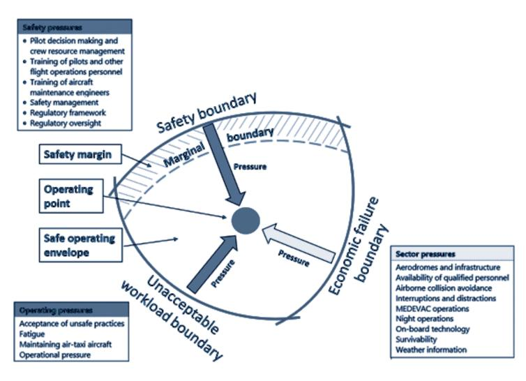
Figure 4. The safe operating envelope model adapted for this SII. (Source: TSB)
