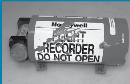
FDR CSMU (above). FDR electronic board (right).
