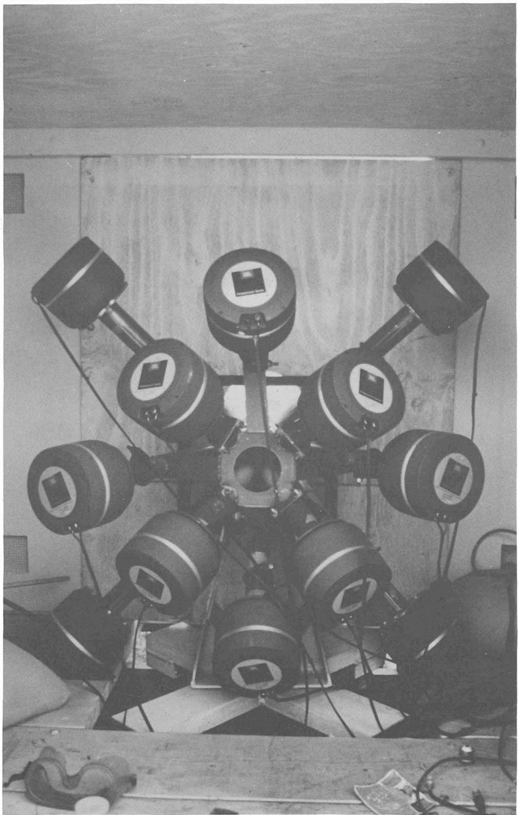
FIGURE 5. Dulles Main Transmitter Manifold Showing 12 Transducers. The manifold is attached to the entry cone of the horn reflector antenna.
