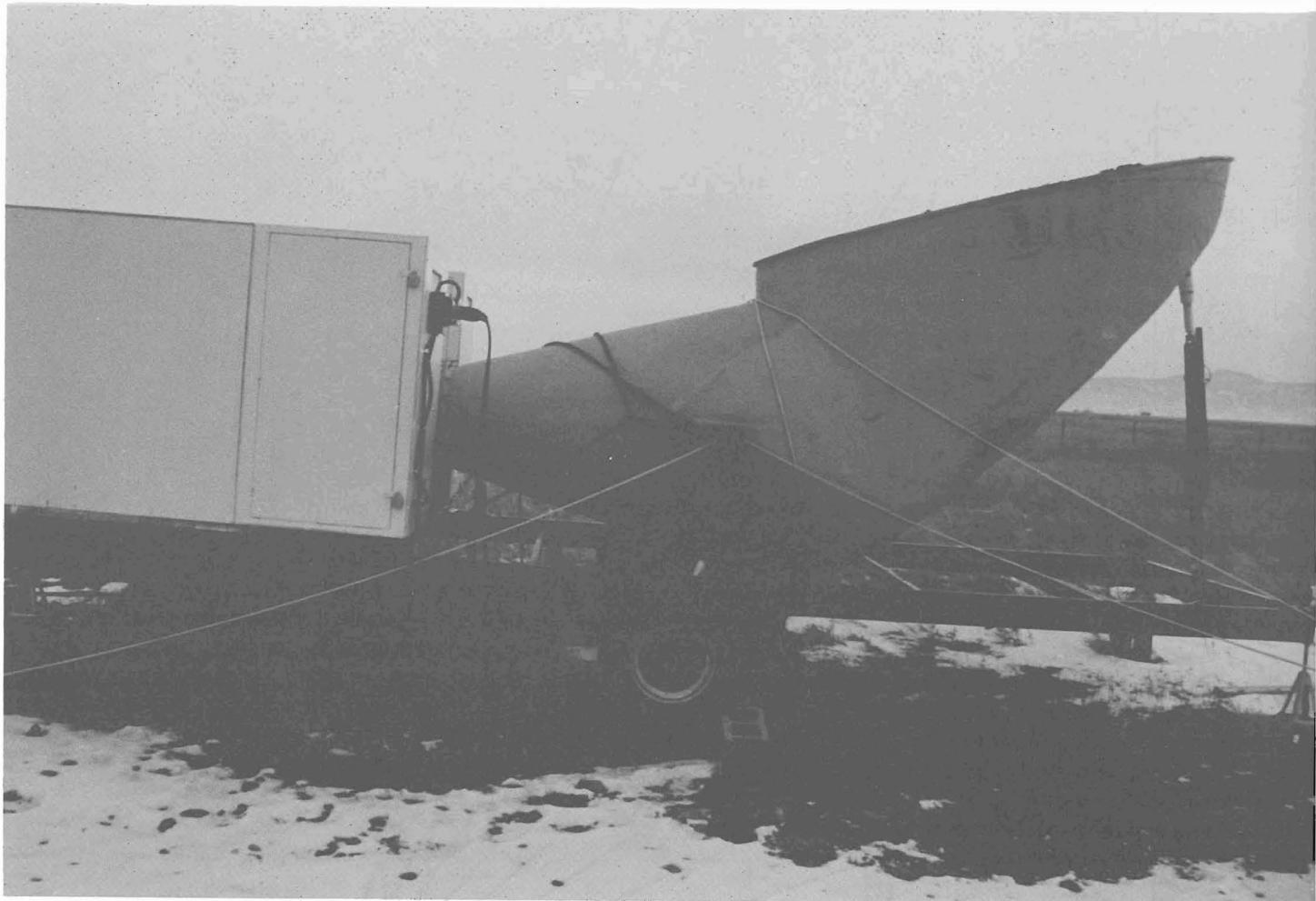
FIGURE 4. Prototype Main Transmitter Mounted on Movable Platform. The diameter of the exit portion of horn is approximately 2 meters.
