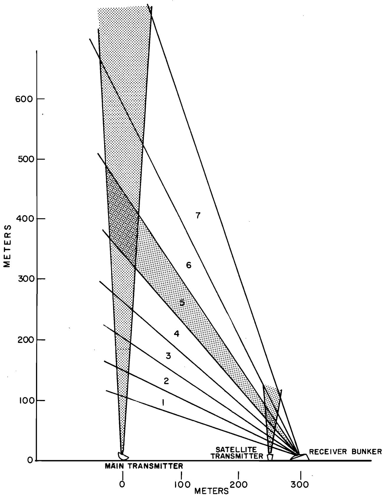
FIGURE 3. Two Dimensional Diagram Showing Intersection of 7 Receiver Beams With Main Satellite Transmitter Beams. Pulses are tracked by switching receiver beams as the transmitted pulse propagates up.
