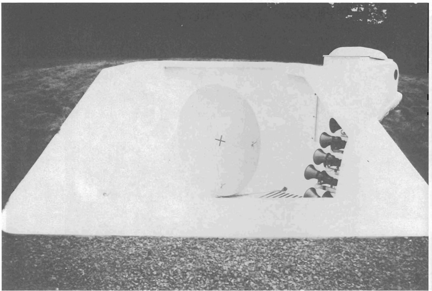
FIGURE 6. Dulles Receiver Bunker Without Cover Showing Acoustic Reflector and Receiver Transducer Array.
